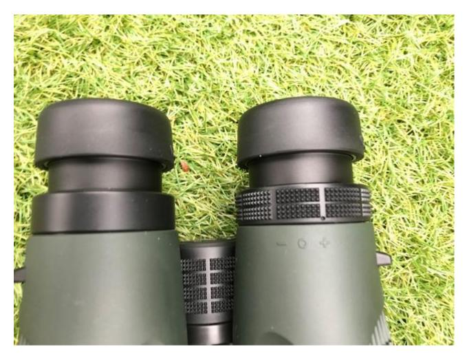
Note the long eye relief on the Series 8 ocular lenses which twist up using three intermediate positions to suit virtually all users.
